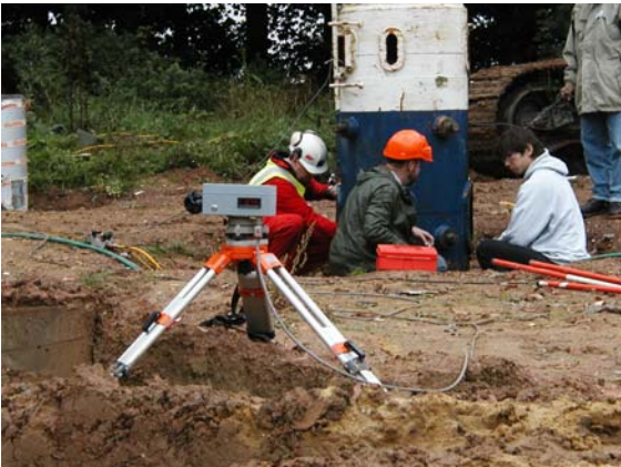
Fig 4. Theodolite in use on Limelette site
