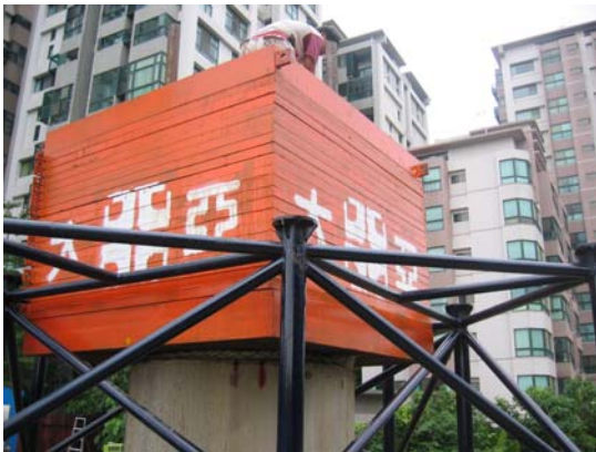
Fig 2. 35 tonne drop mass (Taiwan)
